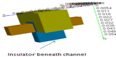
Fig1: buried oxide beneath the channel
